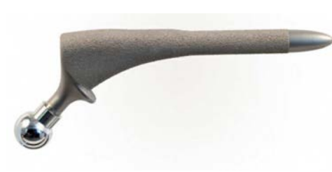
Fig. 2. Endoprosthesis – evaluation of the surface texture of functional (metal) surfaces and the passivated portion (hydroxyapatite)
