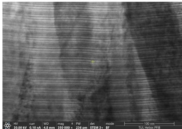
*Fig. 4: STEM image of lamella prepared by PFIB showing AlTiCrN multilayer*
