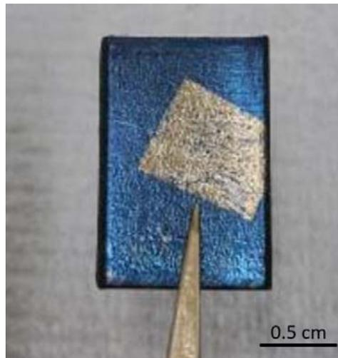
Fig. 2: Graphene used as a thermal corrosion protection layer on the Fe sample.
