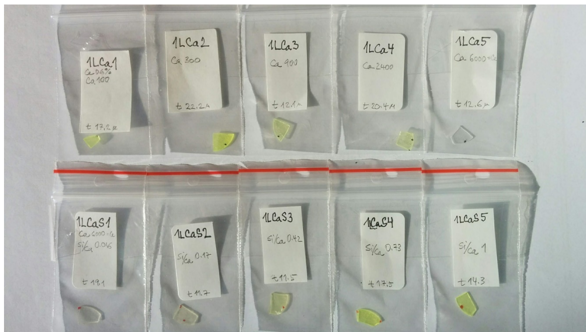
Fig. 1: Color demonstration of the LuAG:Ce,Ca (1LCa) and LuAG:Ce,Ca,Si (1LCaS) specimens. In the 1LCa, the Ca concentration (shown in ppm) grows from left to right; in the 1LCaS the Si/Ca concentration ratio grows from left to right.
