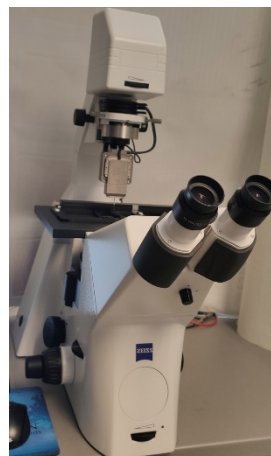
Fig. 2: In-situ indenter BioSoft - Axio Observer3
